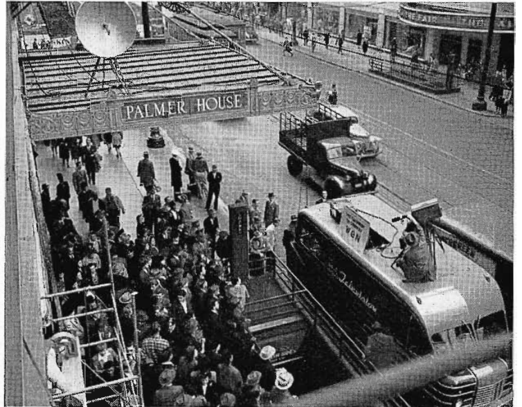
FIG. 10. Another camera, mounted on RCA Mobile Unit, was used to pick up crowds at hotel entrance. Note relay transmitter on marquee. It was used to send convention pickups to WBKB for on-air telecasts.
