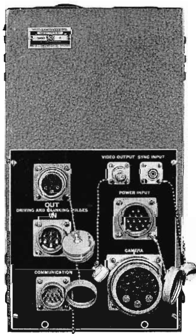
FIG. 6. (Left) This view of the rear of the camera control unit shows how the power and interconnections are made by means of standard plugs and receptacles. All necessary cables, complete with connectors, are furnished. Power and intercom cables are shielded multiple-conductor cables using synthetic insulation and jackets. Video connections are made by means of flexible coaxial cables of standard types having polyethylene cores and vinyl jackets as developed for military use during the war. The camera cable is a special cable containing three 50-ohm coaxials and twenty-one other conductors each of seven strands of #30 gauge copper wire. This cable has an overall shield and a neoprene jacket with an outside diameter of 0.940 inch. It is extremely flexible, small, and light in weight compared with any previous equivalent camera cable. The weight-per-foot is 0.4 lb. It is available in standard lengths of 50, 100 and 200 feet, each fitted with matching connectors.
