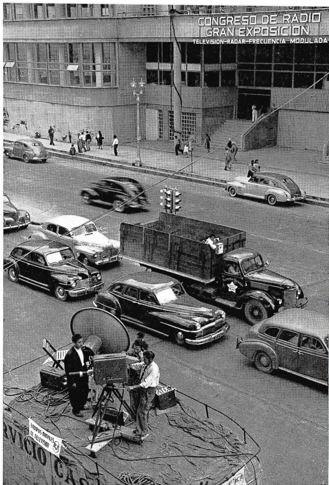
FIG. 5. (Right) Bullfight pictures from the Plaza Mexico, seven miles away, were transmitted to the hotel exposition area by standard RCA Microwave Relay Equipment. In this picture the relay equipment, flown in from New York for the occasion, is being tested before transportation to the Plaza. Note transmitter parabola on the truck and receiver parabola on the hotel parapet. Immediately following this test the transmitter was moved to the Plaza and the receiver to the hotel roof.
