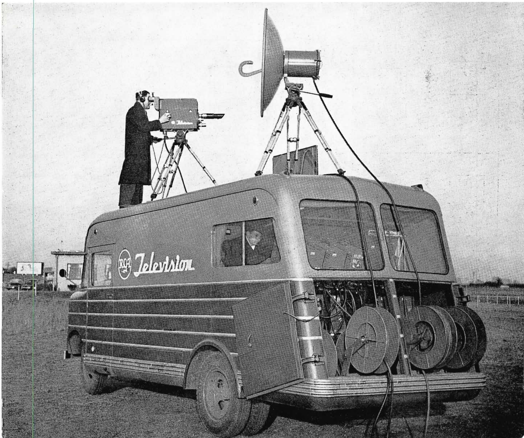
FIG. 3. (Below) This television mobile unit, especially developed to transport the field equipment, is now available as a standard equipment item. The rear part, glass enclosed, is designed for convenient mounting of operating units (see illustration on opposite page).
